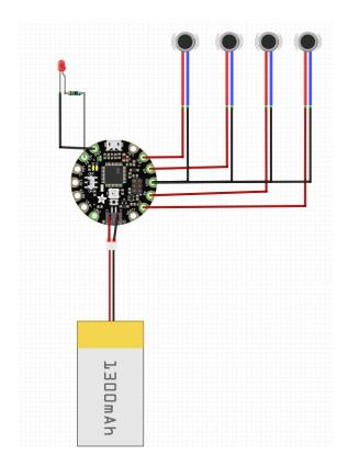
Using the Flora presented a few challenges, first, the Flora only uses 3V, which meant I have manage the circuit in a way that suits a 3V power supply. Second, the Flora only has 4 clear pins for output and one extra pin named SCL, which can be repurposed to use as an output pin.
